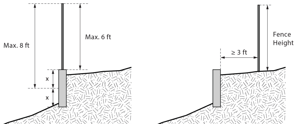
Figure 17.64.030.D-1: Fence and Retaining Wall Combinations
