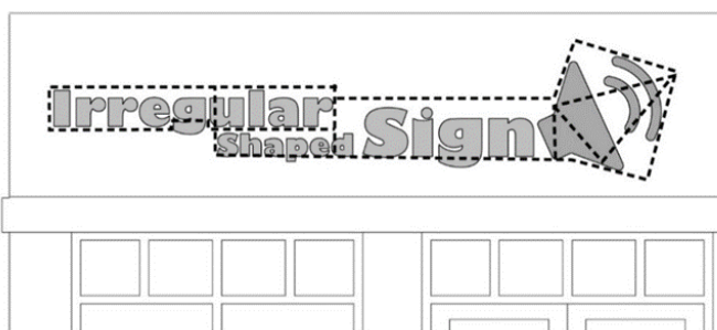
FIGURE 17.72.040.G-3: IRREGULAR SHAPED SIGNS
