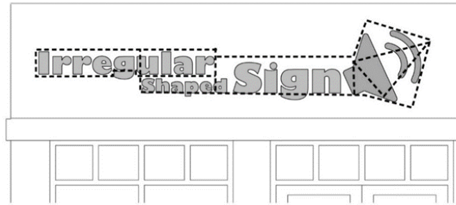
Figure 17.72.040.G-3: Irregular Shaped Signs
